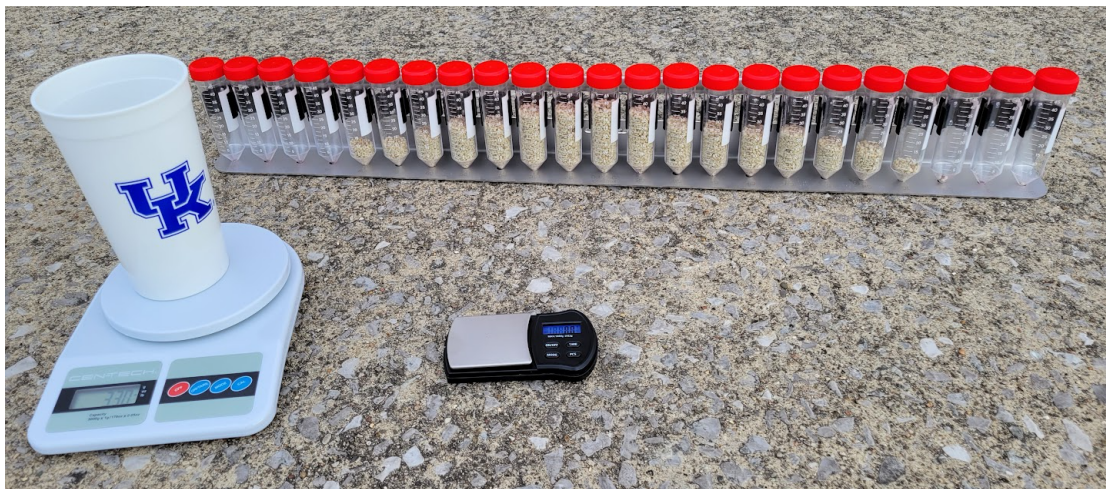
Figure 3. Examples of graduated cylinders and inexpensive scales that could be used to measure the amount of material collected in each pan.
