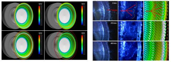
Figure 5: CFD simulation of trajectory of water ligaments and droplets ejected from a rotating spray cup (left), and the measured and calculated liquid surface structure (right).
